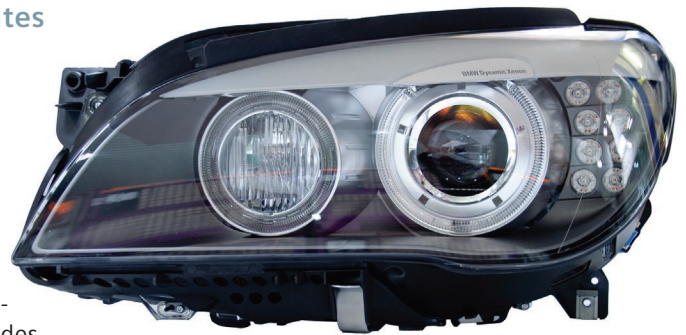
Lighting system with BendLite Xenon cornering light module, ring-shaped daytime driving and position lights and LED turn indicators. Photo: ZKW.
